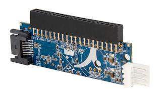
This IDE to SATA adapter converts a 40-pin IDE connector to a SATA connector, allowing you to connect a 2.5in or 3.5in SATA (SATA, SATA II/SATA 300) drive to the motherboard in place of an IDE drive.
